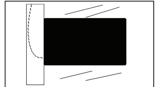
Adhere the backing label to the opposite side of the glass to hide the back of the Surface Mount and iPad.
