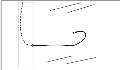
Drill a 3/8" small hole and route the cable down the aluminum channel and out the hole. Make sure there is enough length.
