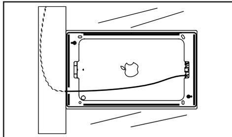
Connect the iPad and place it in the bezel. Attach the bezel to the bracket. Adhere the Surface Mount bracket to the glass close to the channel.
